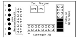
After selection of the appropriate gain links, J2, the system can be fine adjusted and calibrated for fine gain and zero using the multi-turn trimming potentiometers.
